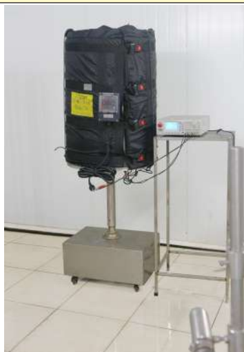
Insulation resistance measurement after IPx6 tests
