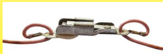
Calor slow-break heating blanket temperature limiter, calibrated at 80°C (circa 1960). Note the waterproof PVC sleeve welded on the wires and the loop made by the electrical conductors passing through a hole in each terminal- this is to eliminate tensile stresses on the wire (Ultimheat Collection)
