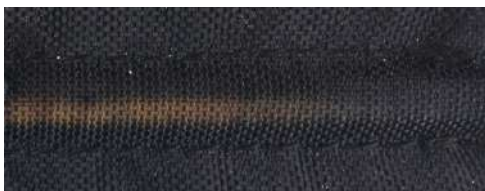
1h at 220°C on the heating cable: the PA66 starts to change color
